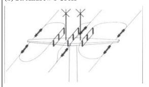
(c) Insulated perch sites lengthwise to the crossarm and acrylic glass rods
