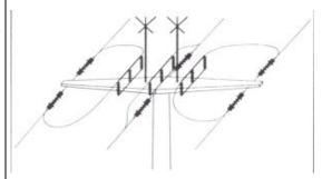
(c) Insulated perch sites lengthwise to the crossarm and acrylic glass rods
