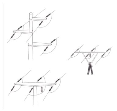
Strain poles with one conductor <a href="mailto:above">above</a> the crossarm.
